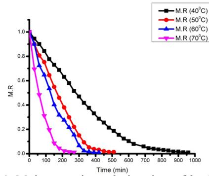
Figure 1. Moisture ratio vs drying time of *kachkal* peel
